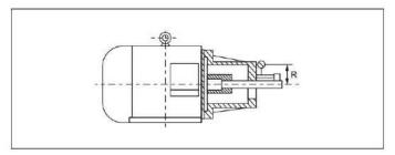
The verticality error is ø0.05 (R is the diameter on the distribution hole of the pump mounting screw hole) pump shaft mounting hole check the vertical mounting angle of the flange
