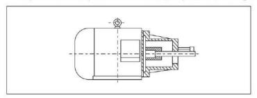
Coaxial error is ø0.05 pump shaft mounting hole on the flange mounting hole coaxial check
